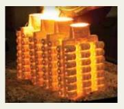
Heat treating alters the physical properties of the metal to produce the desired characteristics: a stronger, tougher and cleaner blade.
