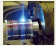
Laser etching uses advanced computer technology to mark each blade for precise identification purposes.
