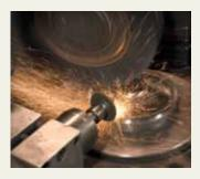
Gear teeth polishing is an important step to ensure that the complementary projections transmit force and motion in the most precise, smoothest manner possible.
