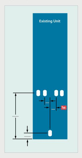
When the risers are going to be reused, the centerline of the unit is the reference point for locating the Supply/Return and condensate connections.
