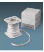
The original form-in-place gasketing, it's the most versatile and cost-effective alternative to sheet gasketing for large equipment flanges. Ideal for sealing complex surfaces, it conforms extremely well to rough or pitted surfaces. It's easy to install, too: just peel off the backing, apply to the surface, and overlap the ends for a remarkably tight seal.
