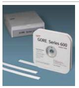
A form-in-place gasket for glass-lined equipment that guards against premature gasket failure. Unlike PTFE envelope gaskets, it won't degrade due to chemical attack, ensuring a tight, long-lasting seal. Made from 100% multi-directionally expanded PTFE, the entire gasket is chemically inert. It conforms to common glass-lined flange imperfections, yet maintains dimensional stability. Plus, installation is quick, easy and lower cost.
